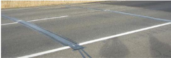
Figure 24 – Single Lane Portable WIM Sensor
