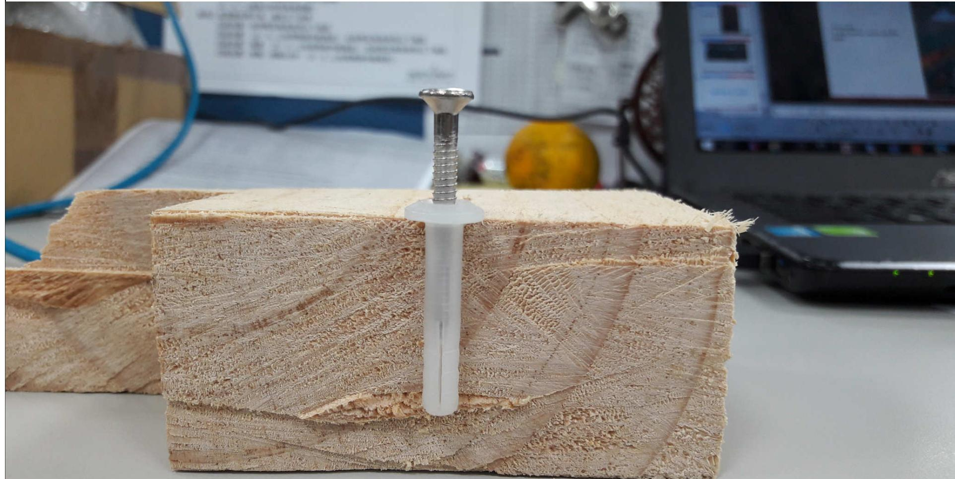
**The screw driving to appropriate depth
