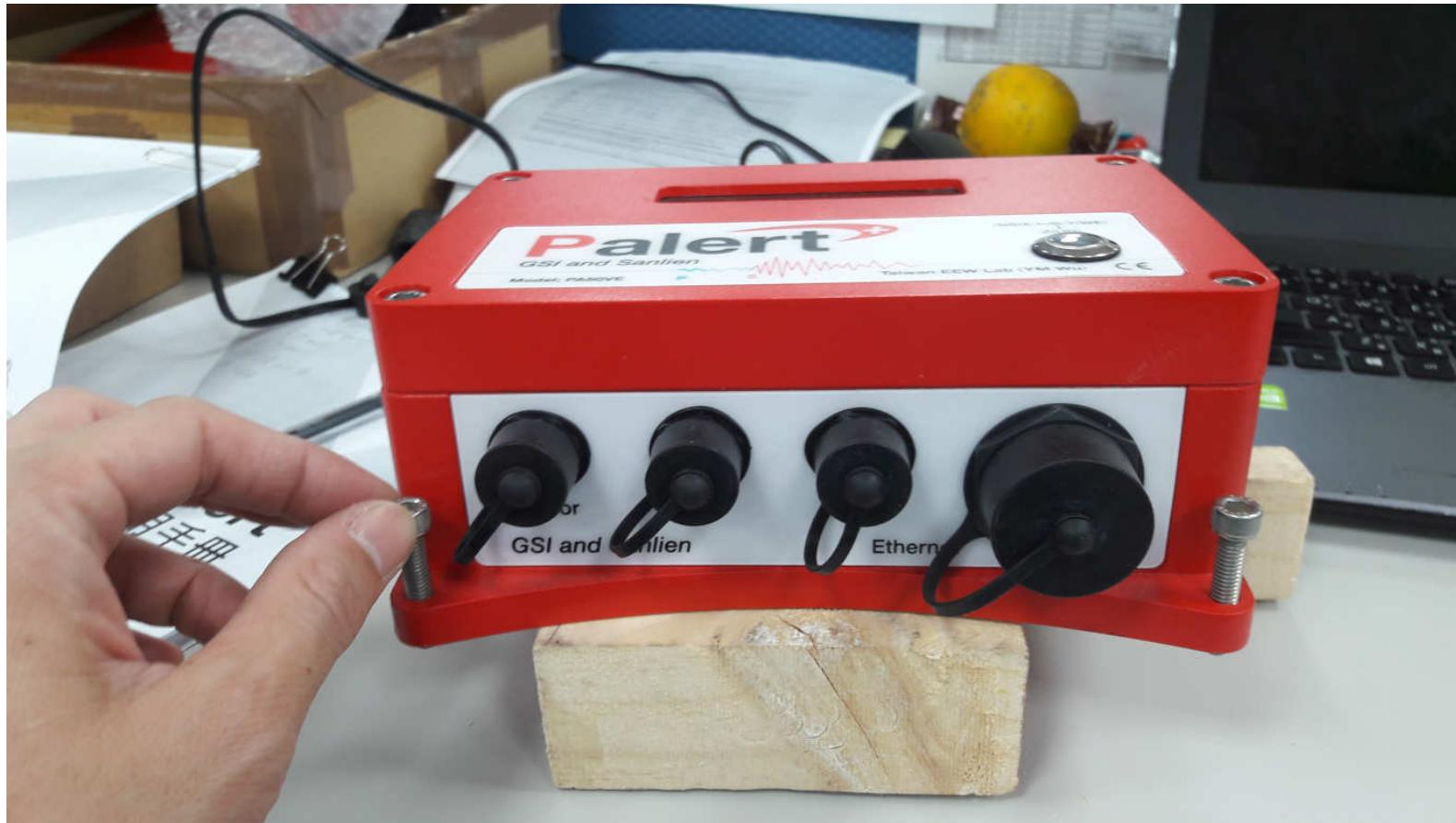
**Leveling 3 of boundary screws approach the platform**
