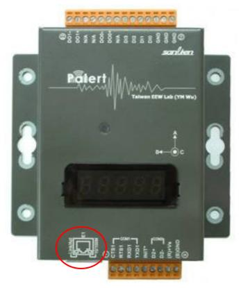
3. 2 sets of D/O and COMS are able to be connected to other devices, such as gas valves, elevator controllers, or through HMI or PLC to control other equipment.
