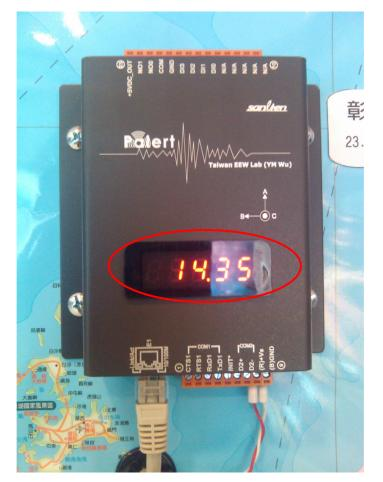
5. When triggered by P wave, the screen shows "P" and P-alert will give estimated maximum intensity 3 seconds after P wave is detected. And because the A axle is designed to detect P wave, P-alert needs to be fixed on a concrete object vertically. Concrete walls or girders on the first floor are good locations. Basements is another perfect sopt for P-alert.
