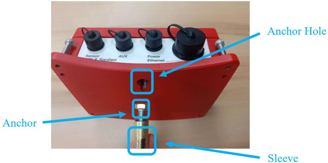
Step 1 : Drilling a hole with sleeve anchor diameter and depth on the wall or platform(ground), diameter and depth around 0.5 and 1.58 inches.
